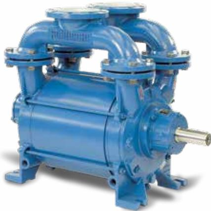
The **RVS** series are liquid ring vacuum pumps and thanks to innovative features, they are able to suck in gas and vapors, without contamination from lubricants, even with dragged fluid and virtually isothermal gas compression. The series can achieve up to 33 mbar (a) and capacity up to 4200 m<sup>3</sup>/h.
